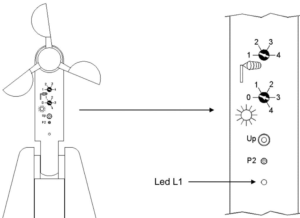
The ref. 5119 controls the roller blind systems exclusively when the wind or the sun exceed the value of thresholds set. For standard controls (i.e. UP or DOWN) of the tubular motors are always required the Mottura handheld or wall remote controls at 433 MHz.
