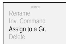
5. Using the “▲”and “▼” buttons select “Assign to a Gr.” and confirm with the “■” button
