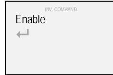
6. Using the "▲" and "▼" buttons select "Inv. Command" and confirm with the "■" button (a tick symbol "✓" appears to confirm the system movement has been inverted)
