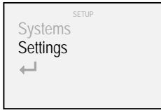
2. Using the “▲”and “▼” buttons select “Settings” and confirm with the “■” button
