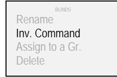
5. Using the "▲" and "▼" buttons select "Inv. Command" and confirm with the "■" button
