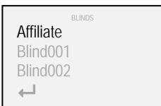
4. Using the “▲” and “▼” buttons, select the system to be deleted and confirm with the “■” button
